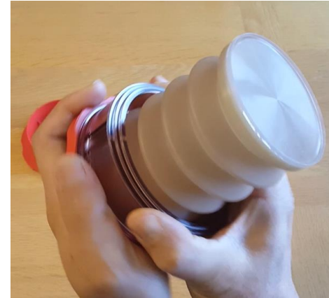
Screw up Press Guide and Pulling Plate, keep them tight...
