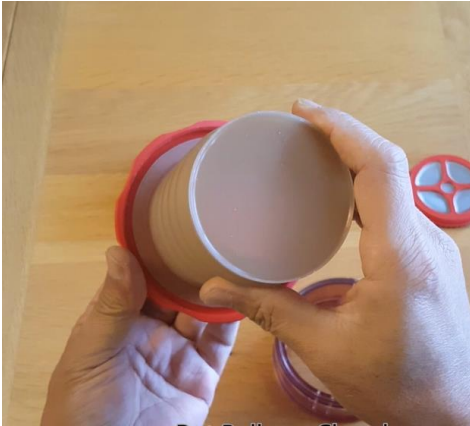
Put Bellows Chamber at the centre of Pulling Plate
