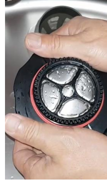
Clean micro-Filter with pump action
