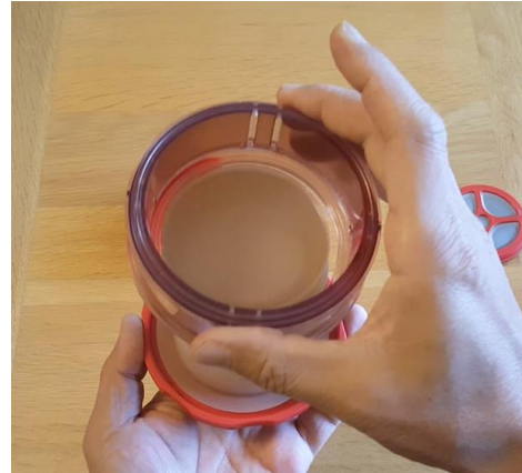
Align Press Guide into Pulling Plate
